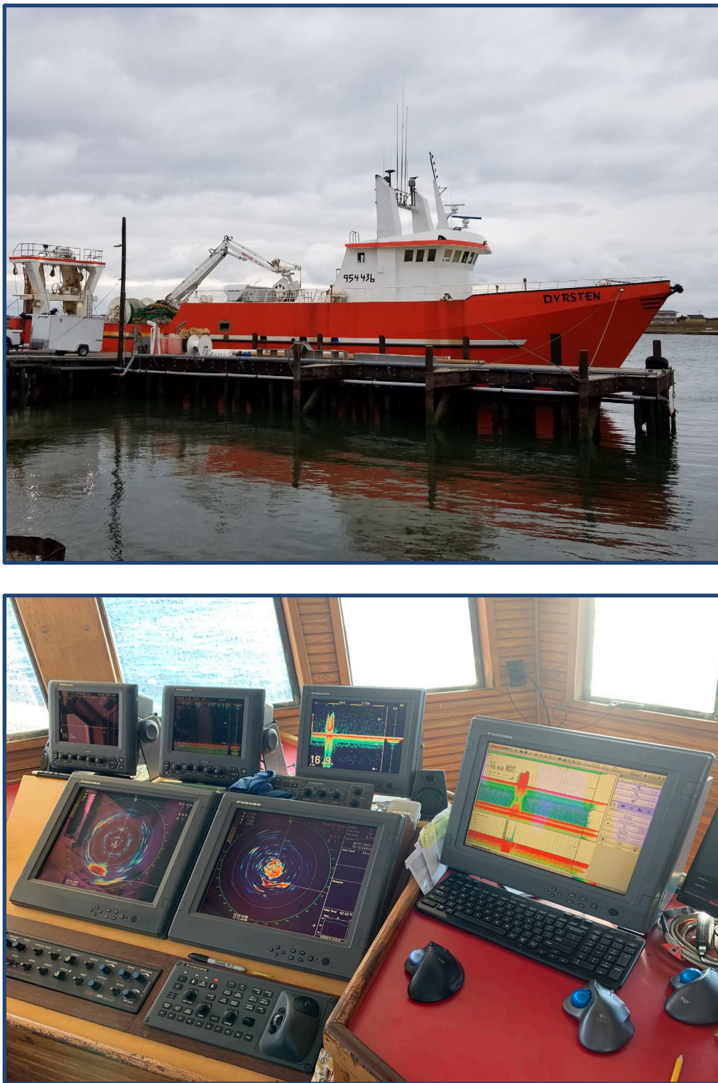
Figure 1-2 (Top) 49-m commercial midwater trawling vessel, F/V Dyrsten , equipped with a recordable 38 kHz Simrad ES80 split-beam echosounder and a Furuno FSV25S omnidirectional sonar. (Bottom) Instrumentation and sonar displays at the helm.
